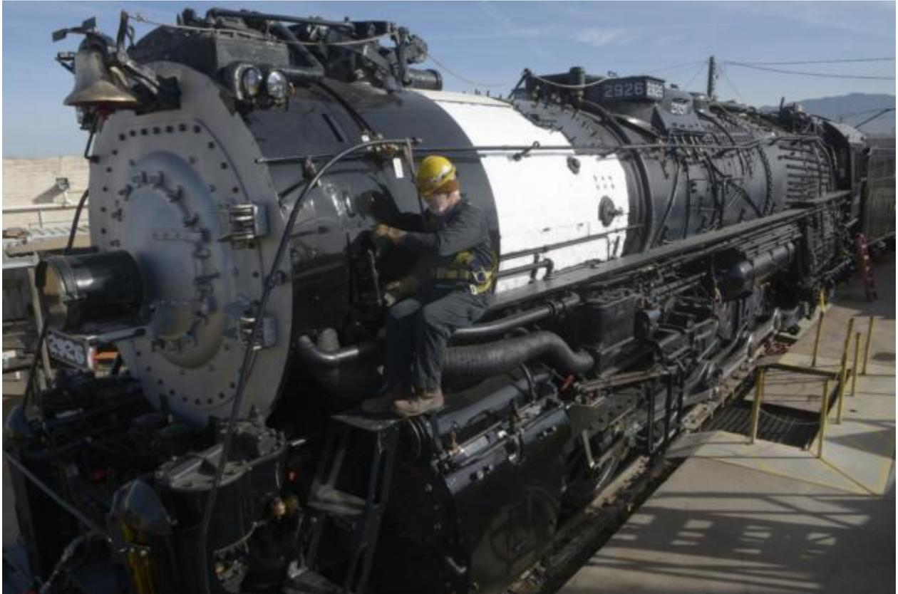
Bill Wilhelm of Placitas checks the fitting of a metal jacketing piece during restoration work on steam locomotive Santa Fe 2926. Members of the New Mexico Steam Locomotive & Railroad Historical Society have been working on the locomotive for more than 15 years. (Greg Sorber/Albuquerque Journal)
