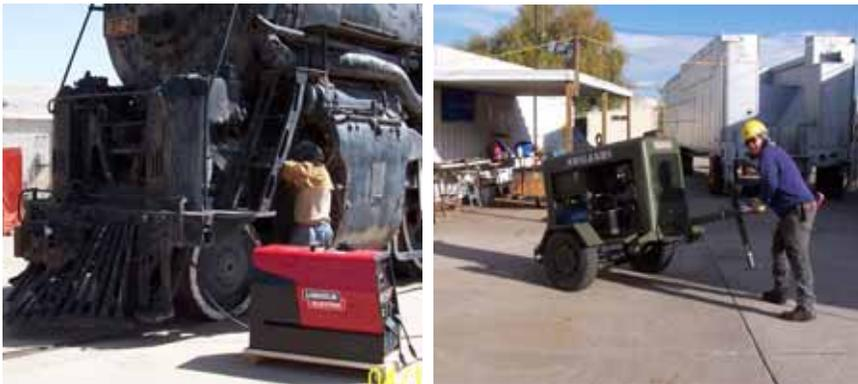
Arc welding units: (Left) The Lincoln unit is now mounted on a steel pallet with rollers, allowing mobility by pushing (on slab or floor) or by forklift. (Right) Old welding unit is powered by a decades old 4 cylinder engine, but it still works.
