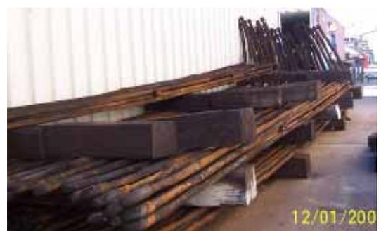
*Superheater pipes stacked alongside a storage container, awaiting refurbishing or replacement.*
