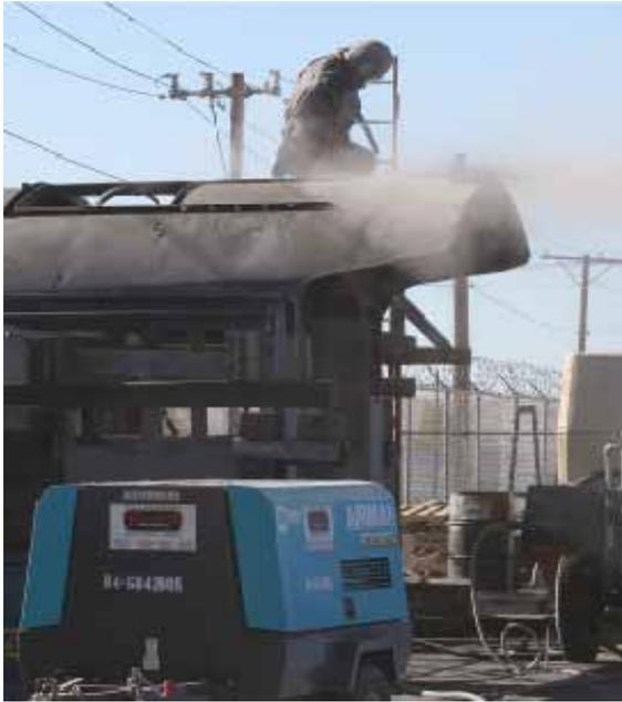
*Above: Recently, R&R was back again. This time they quickly blasted the cab of 2926 free of many years of paint and corrosion.*
