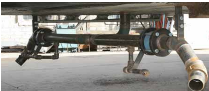
Side pipes and vertical standpipe, (just right of center), complete with check valves and drains and attached to the tender bottom. Only the ends will be visible when tool boxes and trucks are reinstalled.
