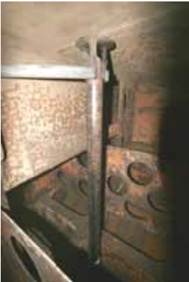
Waterfill standpipe secured inside tender
