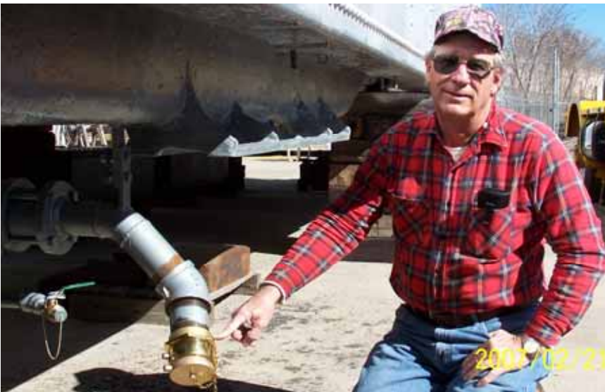
Rick Kirby points to the removable brass coupler that will be used to connect to track-side water sources to the 2926 tender. An identical coupler is on the other side, and a similar fitting is at the rear of the tender to connect to an additional tender.
