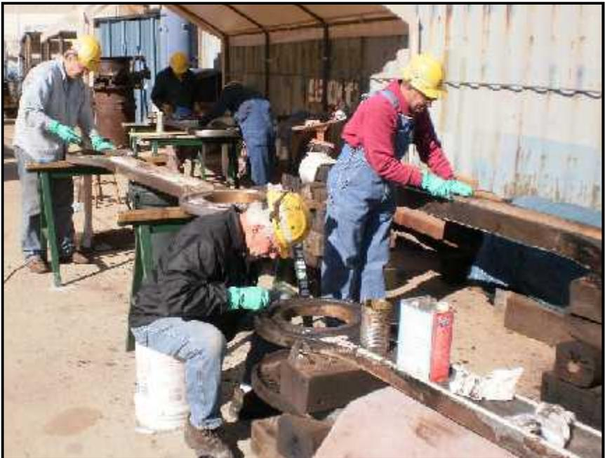
**Busy Bees At A Side Rod Cleaning Party.** *The massive side rods, like all other parts are cleaned, polished and stored to await reinstallation. Meanwhile, their bearings are being thoroughly cleaned, and with guidance from Timken, will undergo a detailed inspection.*
